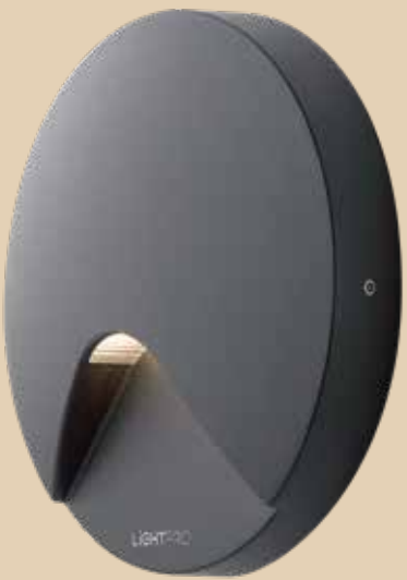
Kuma (184W) Aluminium - Anthracite LED 6 W 3.000 K 300 lm 145 x 35 mm (Ø x D)
